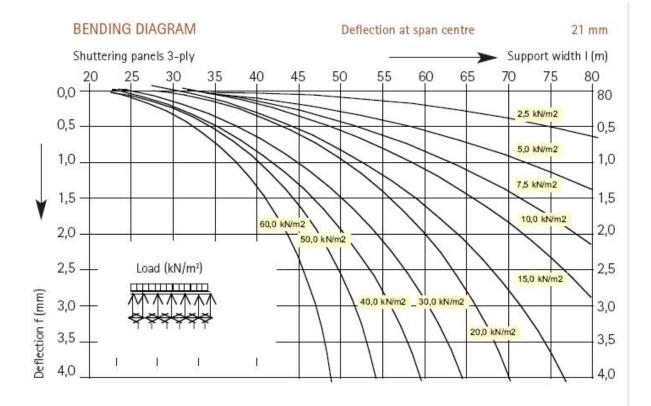
The deflection values were determined in tests after 24 hours of immersion in water. The fibre direction of the cover layers is vertical to the supports.
